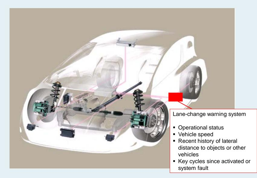
Vision-based lane position warning system (Iteris)
